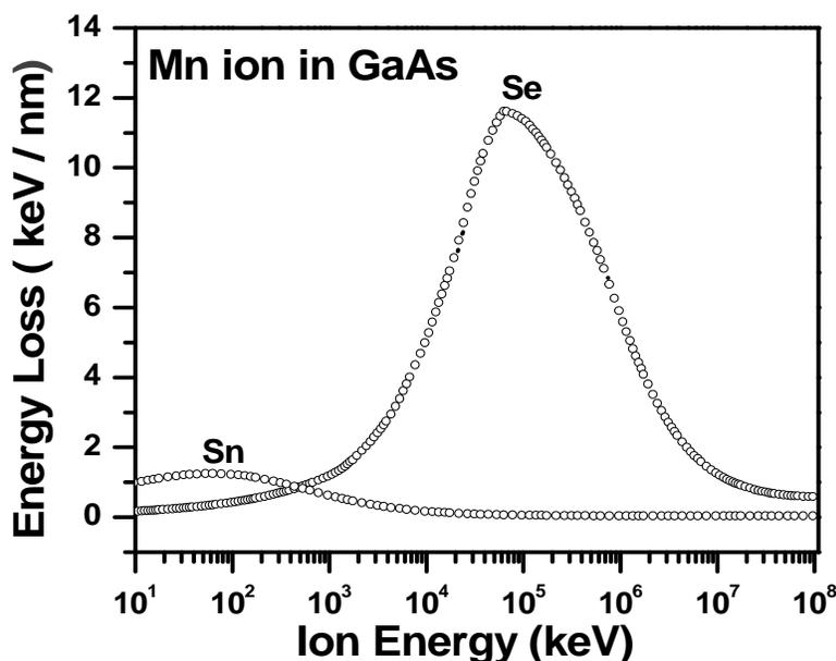
**Figure 1:** Variation of nuclear energy loss and electronic energy loss as a function of ion energy for Mn ions in gallium arsenide.
