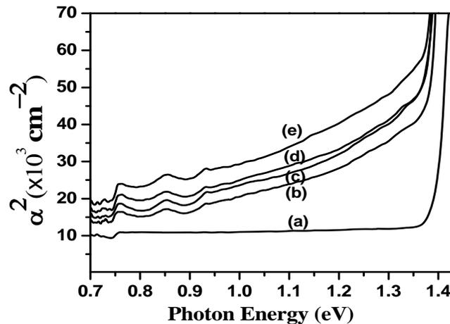
**Figure 4:**  $\alpha^2$  versus photon energy spectra of gallium arsenide; (a) non-implanted and implanted with 325 keV  $\text{Mn}^+$  ions at fluence of (b)  $1 \times 10^{15}$ , (c)  $5 \times 10^{15}$ , (d)  $1 \times 10^{16}$  and (e)  $2 \times 10^{16}$  ions  $\text{cm}^{-2}$ .
