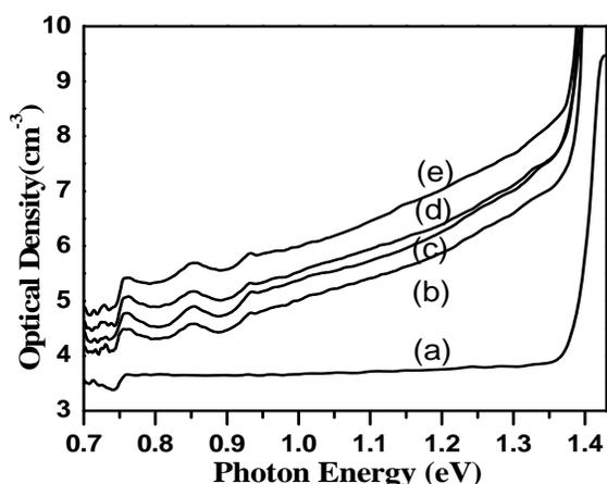
**Figure 5:** Optical density vs photon energy curves of GaAs; (a) non-implanted and samples implanted with 325 keV  $Mn^+$  ions at fluence of (b)  $1 \times 10^{15}$ , (c)  $5 \times 10^{15}$ , (d)  $1 \times 10^{16}$  and (e)  $2 \times 10^{16}$  ions  $cm^{-2}$ .
