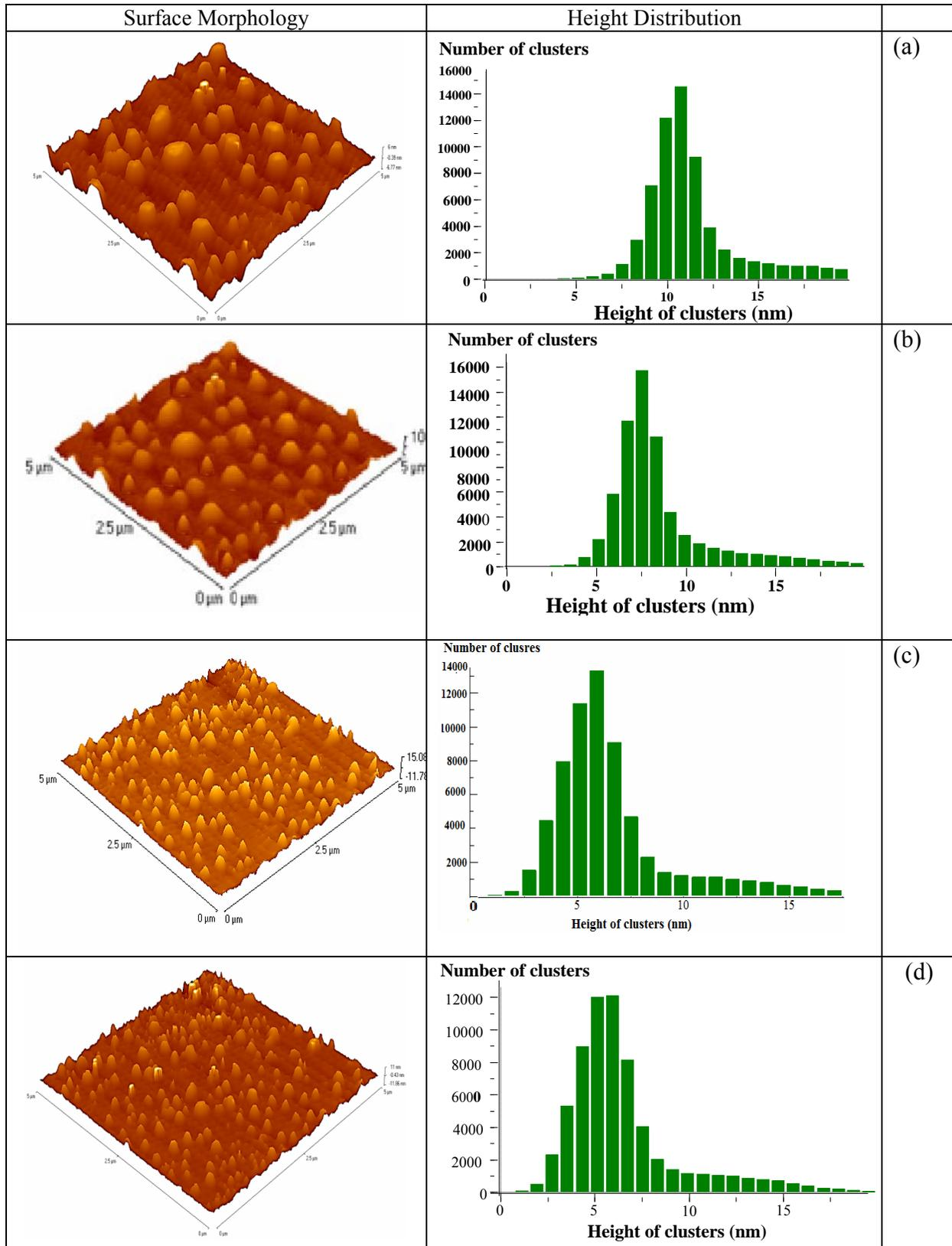
**Figure 2:** Three dimensional AFM images with histograms of GaAs (a) non-implanted and implanted with 325keV Mn ions at fluence of (b)  $1 \times 10^{15}$ , (c)  $5 \times 10^{15}$ , (d)  $1 \times 10^{16}$ , (e)  $2 \times 10^{16}$  ions  $\text{cm}^{-2}$ .
