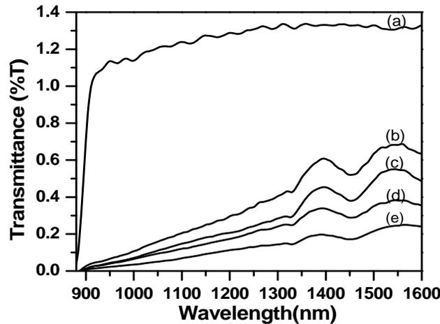
**Figure 3:** Transmission spectra of gallium arsenide; (a) non-implanted and implanted with 325 keV  $\text{Mn}^+$  ions at fluence of (b)  $1 \times 10^{15}$ , (c)  $5 \times 10^{15}$ , (d)  $1 \times 10^{16}$  and (e)  $2 \times 10^{16}$  ions  $\text{cm}^{-2}$ .
