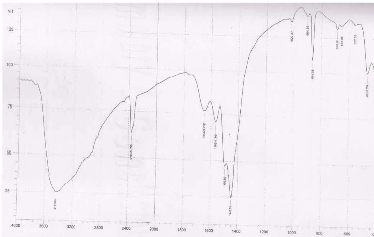
Fig. 3 FTIR of PbO
