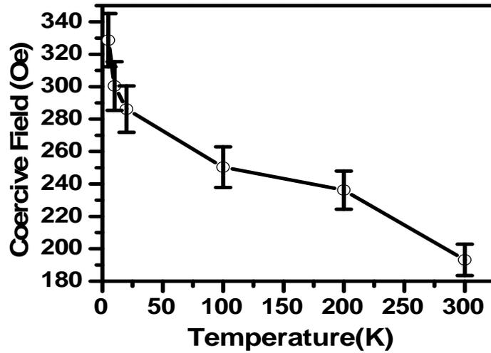
Figure 2. Hc-T Curve Of GaAs +Mn<sup>+</sup> +Si
