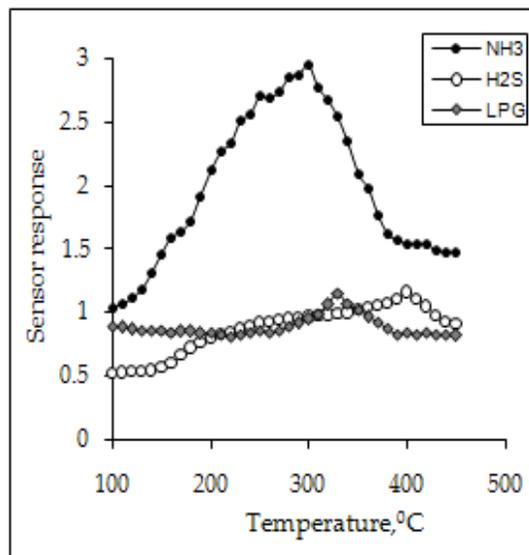
**Figure 5:** Sensor response with temperature of  $\text{WO}_3$  Film for 400 ppm of  $\text{NH}_3$ ,  $\text{H}_2\text{S}$  & LPG.
