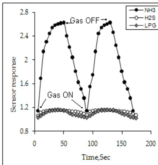
**Figure 6:** Sensor response with response time and recovery time of WO<sub>3</sub>.
