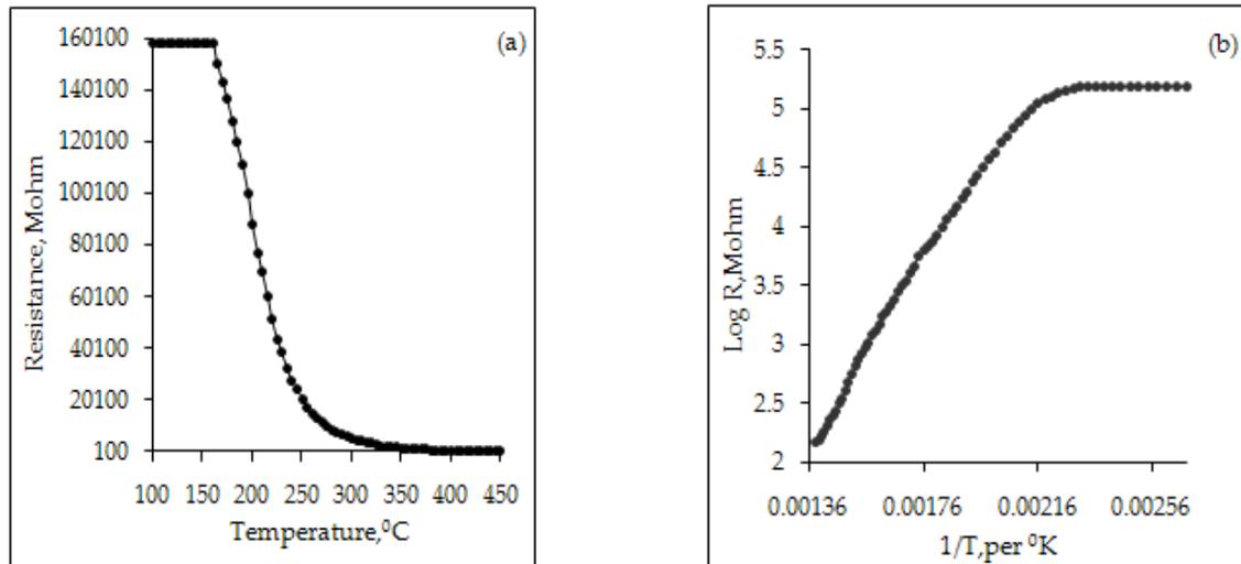
**Figure 4:** Variation of (a) Resistance with temperature fired at  $500^\circ\text{C}$ . (b) Log R Versus  $1/T$  of  $WO_3$  Thick film
