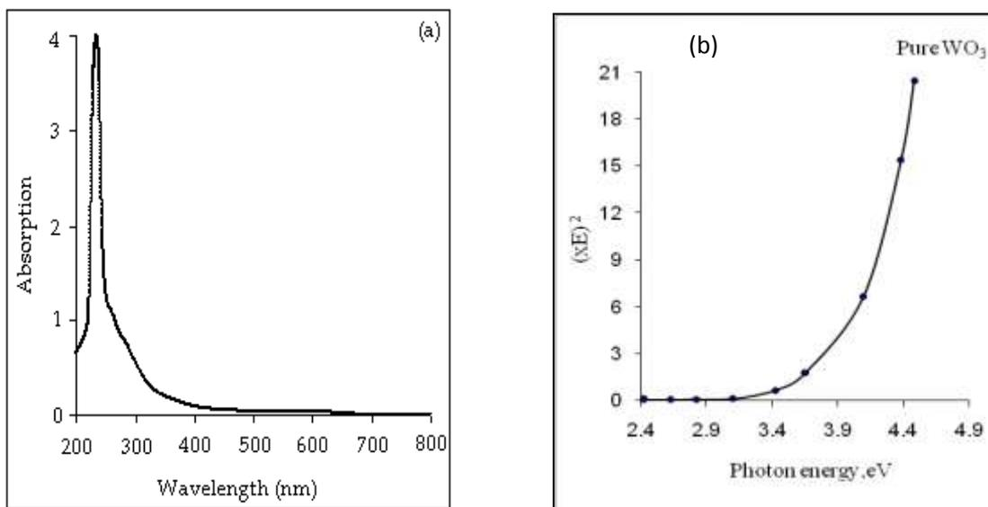
**Figure 3:** (a) Absorbance spectra of WO<sub>3</sub> sintered at 450°C (b) Plots of  $(\alpha h\nu)^2$  against  $(h\nu)$  for WO<sub>3</sub>.
