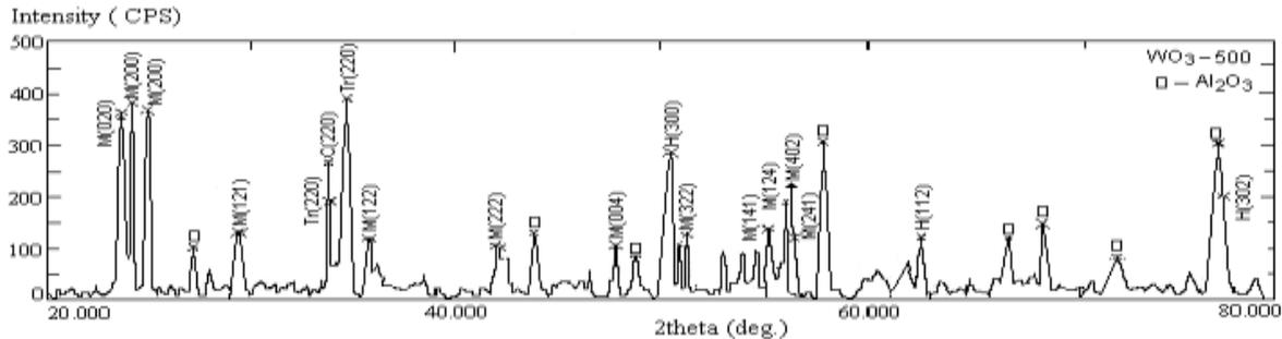
**Figure1:** XRD Pattern of  $WO_3$  Thick film fired at  $500^\circ C$ .
