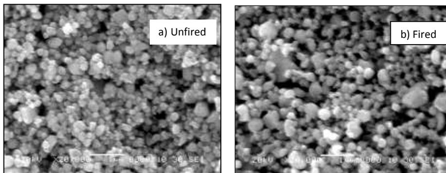
**Figure 2:** SEM image of  $WO_3$  Thick film Fired at  $500^\circ C$ . (a) Unfired  $WO_3$  (b) Fired  $WO_3$
