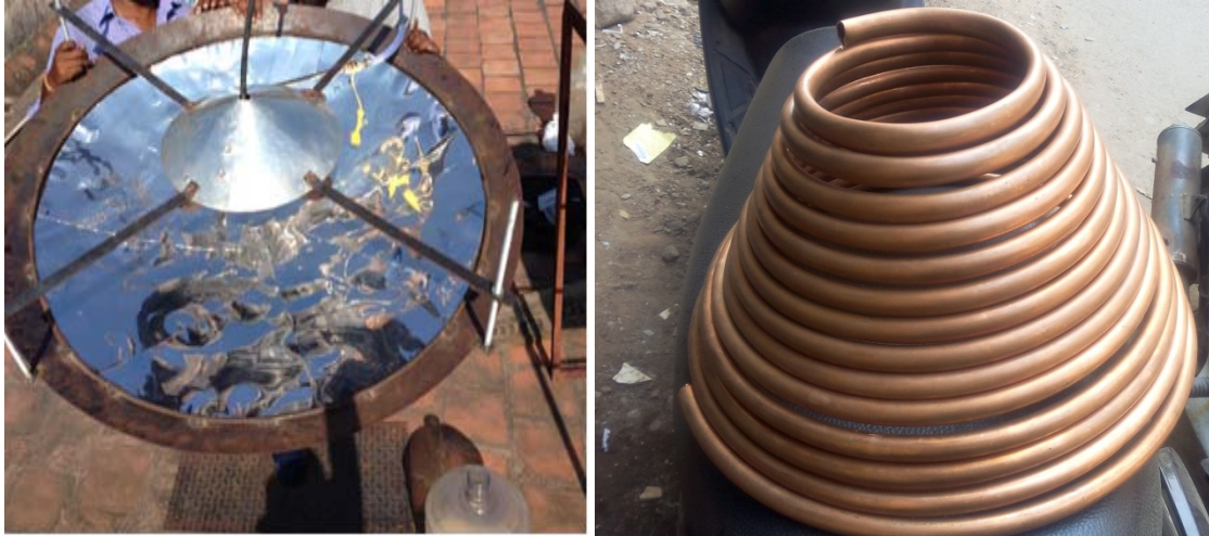
Figure .2 (a) Photographic view of Schematic of Parabolic dish with conical coil setup (b) Receiver coil
