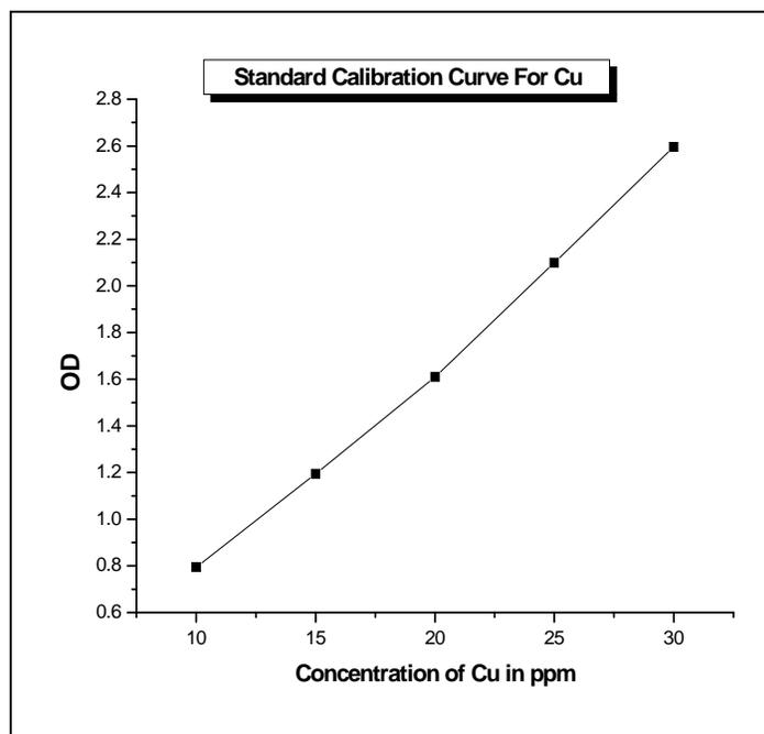
**Figure 1:** Graph of OD Vs Concentration of Copper in ppm
