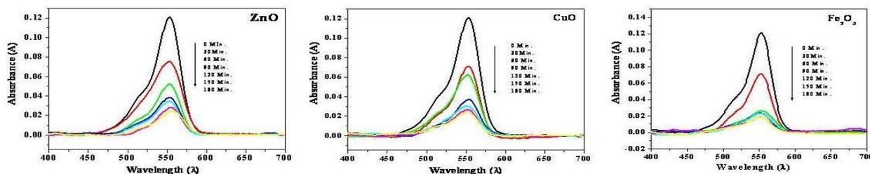
**Typical time-dependent UV-Vis spectrum of Rhodamine B dye in presence of nanoparticles..**
