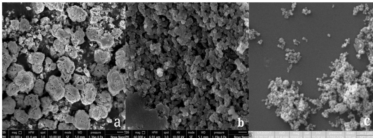
**Fig 2 SEM images of a) CuO b) ZnO and c) Fe<sub>2</sub>O<sub>3</sub> respectively**
