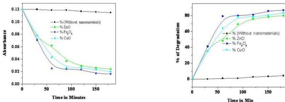
**Typical plot of (a) % degradation versus irradiation time, (b) relative absorption (A/A<sub>0</sub>) versus irradiation time**
