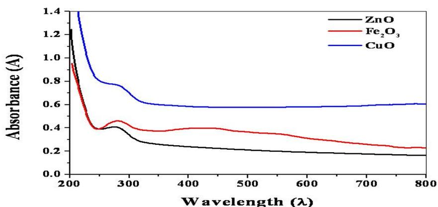
**Fig 1 UV-Visible absorption spectra of the as grown nanoparticles**
