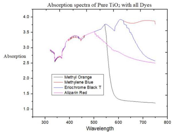
Fig.3: Absorption Spectra of Pure TiO<sub>2</sub> with all 4 dyes (1:1 Ratio)
