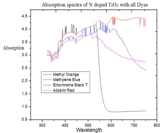
Fig.4: Absorption Spectra of N-doped TiO<sub>2</sub> with all 4 dyes (1:1 Ratio)
