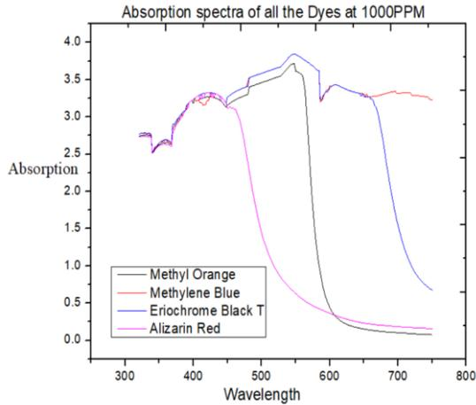
Fig.2: Absorption Spectra of all the 4 dyes
