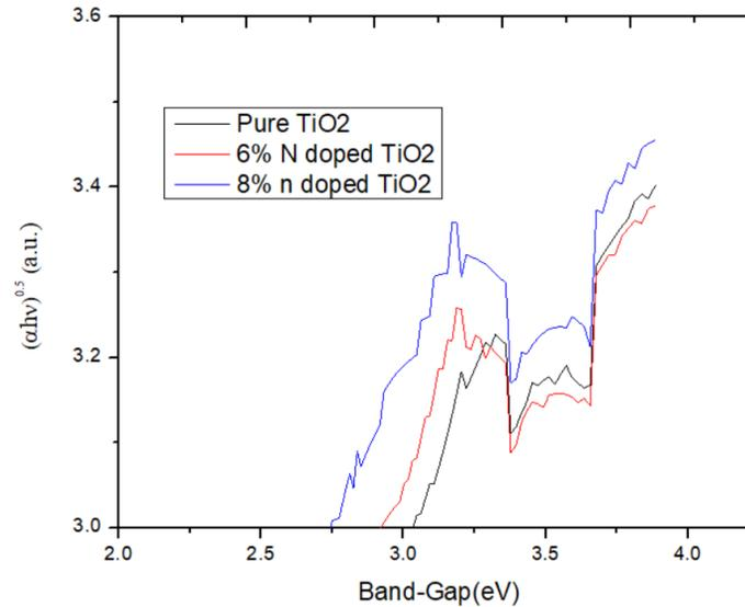
**Fig. 6:** Band-Gap of Pure and N-doped TiO<sub>2</sub>
