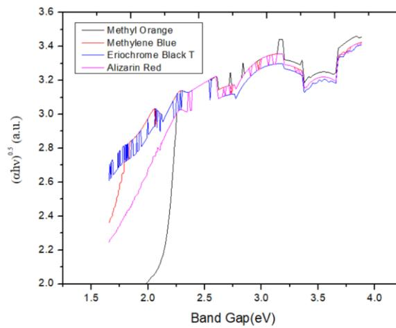
**Fig.8:** Bandgap of 8% N-doped TiO<sub>2</sub> with all 4 Dyes
