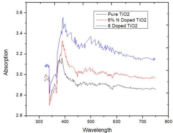
Fig.5: Absorption Spectra of Pure TiO<sub>2</sub> and N-doped TiO<sub>2</sub>
